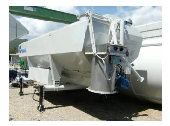
Our silos have roof mounted WAM Reverse Jet air filters to allow the cement to dust to be recycled, 180 degree slewing auger to allow easy positioning of the silo in confined spaces including slewing and adjustable height control loading legs for the quick easy loading and transportation of the Low Level Cement Silo.
